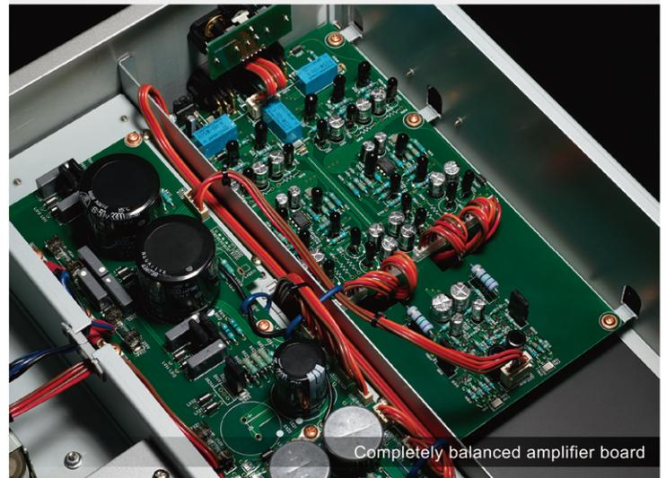
Completely balanced amplifier board
