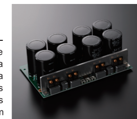
Custom-built large-capacity block capacitor
