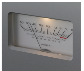
Needle-type meter with electric bulb-colored illumination
